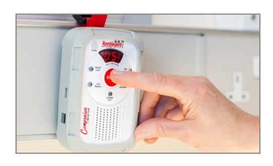
TO DEACTIVATE SLEEP MODE PRESS & HOLD RESET UNTIL LCD SHOWS 'ON'. IT WILL NOW APPEAR AS A BLUE TILE 'TEST PAD' IN ITS STORE LOCATION.
